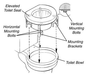
FIGURE 1 - SEAT INSTALLATION/REMOVAL
